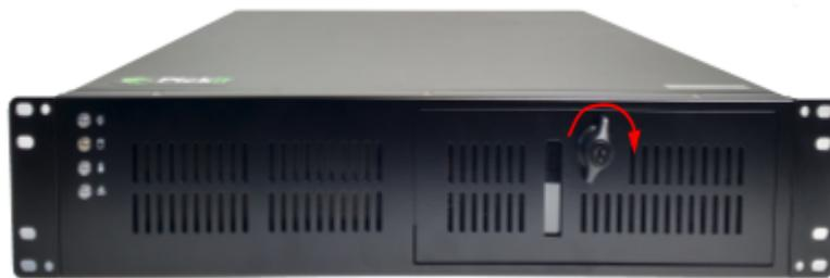
A few ports (which are not used with Pick-it™) and some buttons are located under the lid. The power switch is highlighted by a red circle below. In case of a power failure while the computer is on, it will restart automatically when power is restored.
